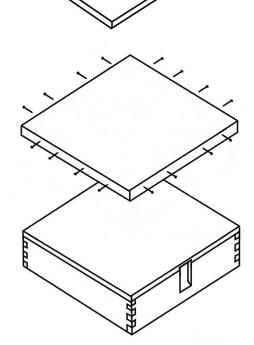
4. Turn top board over and glue and nail to the frame created, using 1" nails, ensuring board vents line up with vents in side walls.
